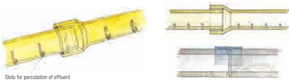
Slots for percolation of effluent
