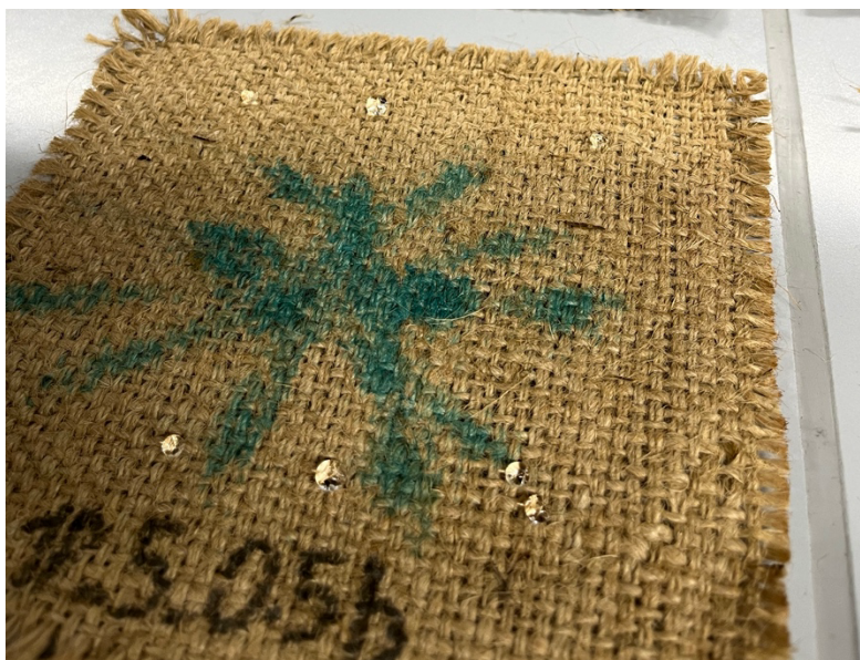
Figure 1: A jute sample demonstrating hydrophobicity due to treatment with Layer-by-layer technology (image source: SUPSI)
