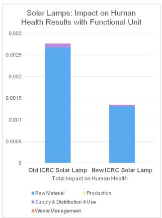
By improving the durability of key components, such as the battery, and doubling the lifespan of the solar lamp, the environmental impact is linearly reduced when evaluated against the function of providing household lighting for the same duration.
